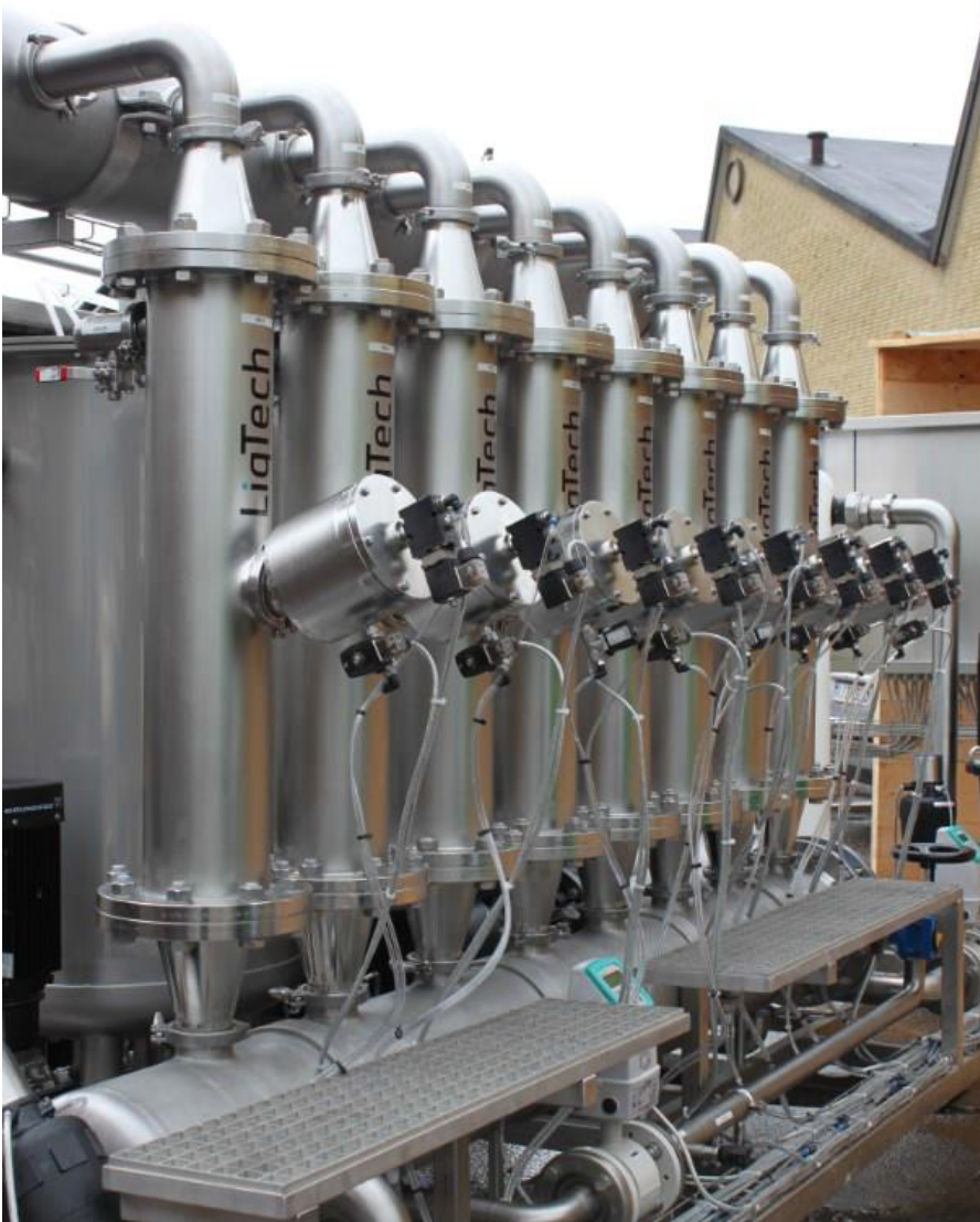
Photo of a system for UF filtration, (photo courtesy of LiqTech).
