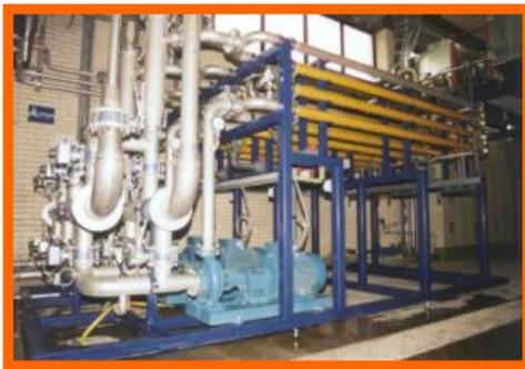
*Membrane unit at a paper-mill plant*
