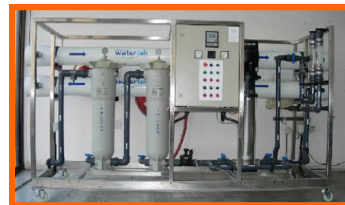
Brackish Water Reverse Osmosis Desalination System; Nominal Capacity: 30.000 gallons/day
